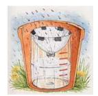
To prevent the rain gauge from blowing over, place it outside in a heavy flowerpot. Alternatively, you could dig a hole in the ground for it to stand in. Make sure the rain gauge is placed in an open area. If it is near any trees or buildings, extra water could drip into it and your measurements will not be accurate.
