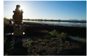
A groundwater monitoring well in Colusa County, north of Sacramento. (Source: California Department of Water Resources)
