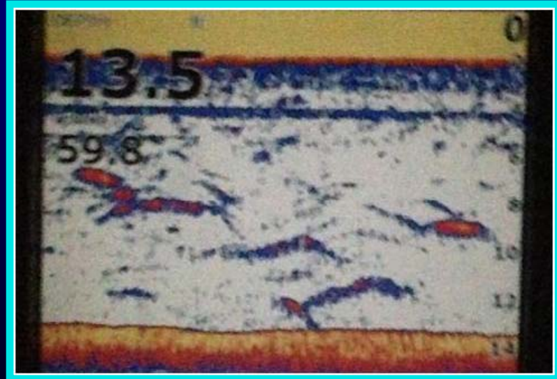
Sonar Image of Striped Bass in Front of a Fish Screen at Night (Dave Jacobs Photo)
